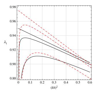
**Figure 6.** Edge (solid) versus body (dashed) bifurcation curves for a thin incompressible elastic plate resting on a local foundation with stiffness  $\kappa = (h/\ell_s)^4 \mu k$  proportional to the wavenumber k and relative compliance  $h/\ell_s = 0, 1/3, 1/2$ , in a state of bi-axial pre-stretch ( $\lambda_1 < 1, \lambda_2 = 1.05$ ). Body wrinkling takes place in compression and always prior to edge wrinkling. (Online version in colour.)
