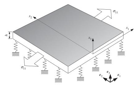
**Figure 1.** Hyperelastic semi-infinite plate resting on a Winkler foundation. Here the plate has been homogeneously pre-stretched along  $x_1$  (equilibrium configuration) by the application of a uni-axial stress  $\sigma_{11}$ .
