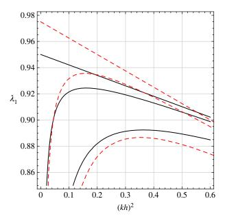
**Figure 5.** Edge (solid) versus body (dashed) bifurcation curves for a thin incompressible elastic plate resting on a Winkler foundation with relative compliance  $h/\ell_s = 0$ , 1/3, 1/2 in a state of bi-axial pre-stretch ( $\lambda_1 < 1$ ,  $\lambda_2 = 1.05$ ). Body wrinkling takes place in compression and parallel to the edge (i.e.  $n_2 = 0$ ); it occurs prior to edge wrinkling for  $h/\ell_s = 0$  and 1/3 and after it for  $h/\ell_s = 1/2$ . (Online version in colour.)
