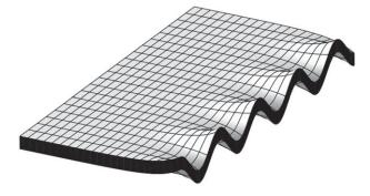
**Figure 2.** Buckling wrinkles with wavenumber k localized near the edge of a compressed thin plate with thickness h.
