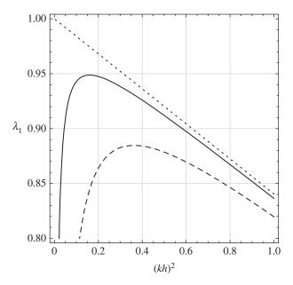
**Figure 3.** Bifurcation curves for the appearance of edge wrinkles with scaled wavenumber kh on a thin plate made of incompressible elastic material with flexural rigidity D, resting on a Winkler foundation with elastic modulus  $\kappa = 3\ell_s^{-4}$ D. The curves are for uni-axial pre-stress and foundation relative compliance  $h/\ell_s = 0$  (dotted), 1/3 (solid) and 1/2 (dashed). In the first case (no Winkler foundation), the plate buckles as soon as it is compressed laterally.
