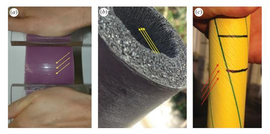
**Figure 1.** Creases appearing in the large deformation of soft matter, as indicated by arrows. (*a*) Large bending of a silicone block with two ends glued to plastic plates, on which bending moments are applied; (*b*) everted tube of pipe insulation material; (*c*) twisted cylinder, on which axial and circumferential lines were drawn prior to the twist. Note how all creases are aligned with a principal direction of stretch.
