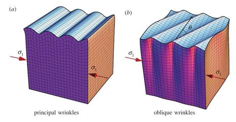
**Figure 2.** Graphical representation of *principal* (*a*) and *oblique* (*b*) wrinkles on the free surface of a compressed semi-infinite soft solid subject to a uniaxial compression with unique Cauchy stress component  $\sigma_1$ . (Online version in colour.)
