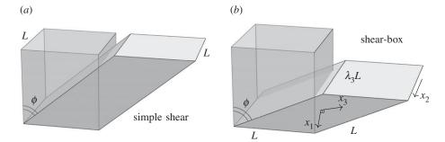
**Figure 3.** Two shearing deformations and their tilting angle  $\phi$  of a soft solid initially occupying a cube of side *L*. (*a*) *Simple shear*, where the top and the bottom faces move on parallel planes. (*b*) *Shear-box*, where the initial front and back square faces become rhombic. In the latter case, two of the Eulerian principal directions are aligned with the diagonals of the rhombi.
