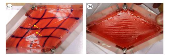
**Figure 5.** (*a*) Freshly solidified gelatin tends to exhibit surface creases instead of sinusoidal wrinkles when subject to an extreme deformation, see arrows. (*b*) Here, the gelatin was left overnight to solidify and a stiffer layer/skin formed on the surface on top of the soft substrate; when deformed, the coated block produced sinusoidal wrinkles.
