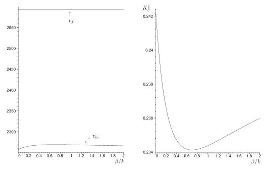
Fig. 4. Influence of an asymptotically homogeneous profile on the wave speed (free and metalized boundary conditions) and on the electromechanical coupling coefficient.
