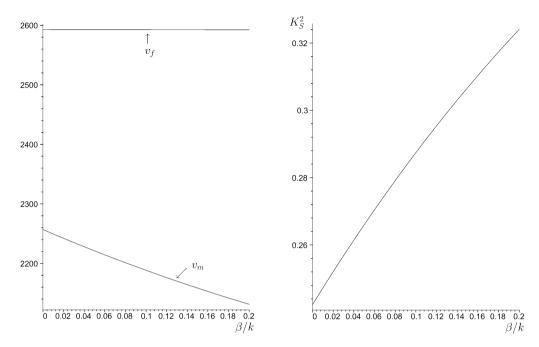
Fig. 1. Influence of a decreasing exponential inhomogeneity function on the wave speed (free and metalized boundary conditions) and on the electromechanical coupling coefficient.
