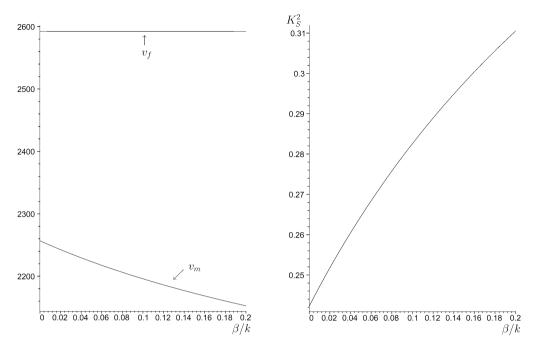
Fig. 2. Influence of an inverse quadratic inhomogeneity function on the wave speed (free and metalized boundary conditions) and on the electromechanical coupling coefficient.
