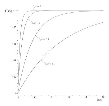
Fig. 3. Variation of an asymptotically homogeneous profile with depth for four different values of the dispersion parameter  $\beta/k$ .
