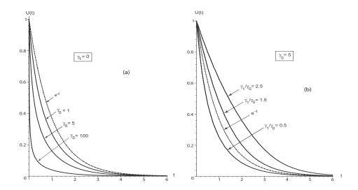
Fig. 3.1. Time recovery function when  $\theta = \pi/2$ : (a)  $\gamma_1 = 0$  and  $\gamma_0 = 1$ , 5, 100; (b)  $\gamma_0 = 5$  and  $\gamma_1 = 0.5$ , 1.5, 2.5. The recovery function for an isotropic solid is also plotted (dotted curve).
