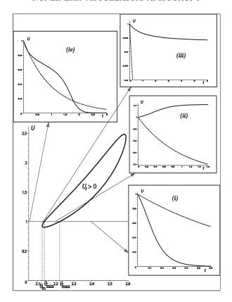
Fig. 3.3. Types of time recovery functions for  $\gamma_0 = 20$ ,  $\gamma_1 = 1$  (strong elastic anisotropy). The amount of shear U starts at 1 for t = 0. Outside the oval shape,  $U_t < 0$  and U decreases as in (i) and (iv): decay toward zero; and in (iii): decay toward a value > 0. Inside the oval shape,  $U_t > 0$  and U increases as in (ii): growth toward a value > 1. The recovery function  $e^{-t}$  for an isotropic solid is also plotted (dotted curves).
