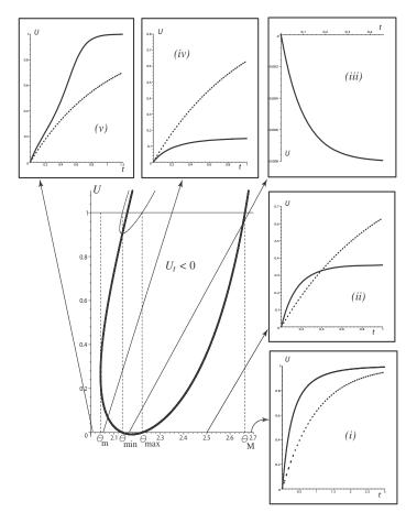
FIG. 4.1. Types of time creep functions for  $\gamma_0 = 20$ ,  $\gamma_1 = 1$  (strong elastic anisotropy). The amount of shear U starts at 0 for t = 0. Outside the thick-line shape,  $U_t > 0$  and U increases as in (i) and (v): growth toward 1, and as in (ii) and (iv): growth toward a value below 1. Inside the thick-line shape, U decreases as in (iii): decay toward a negative value. The creep function  $1 - e^{-t}$  for an isotropic solid is also plotted (dotted curves).
