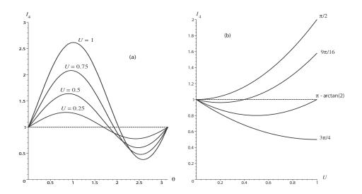
FIG. 2.1. Variations of the squared stretch in the fiber direction: (a) with the angle and (b) with the shear. When  $I_4 > 1$ , the fibers are in extension; when  $I_4 < 1$ , they are in compression.
