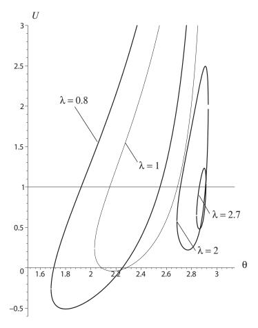
Fig. 4.2. Effect of prestretch on time creep functions for  $\gamma_0=30,\ \gamma_1=1$  (strong elastic anisotropy). The amount of shear U starts at 0 for t=0. Inside the thick-line shapes, U decreases; this situation may arise when the solid is not prestretched ( $\lambda=1$ ) or when it is compressed ( $\lambda=0.8$ ). Outside the thick-line shapes,  $U_t>0$  and U increases; this situation may arise when the solid is in extension ( $\lambda=2,\ \lambda=2.7$ ).
