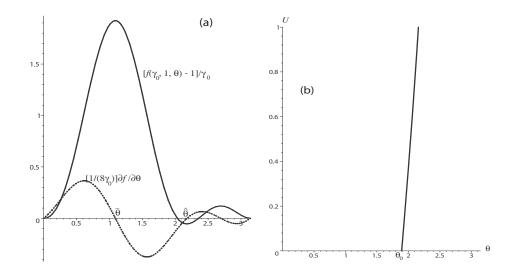
FIG. 5.1. (a) Variations with  $\theta$  of  $[f(\gamma_0, 1, \theta) - 1]/\gamma_0$  and of its derivative, showing an absolute minimum at  $\hat{\theta} = 2.1777$ . (b) Variations of  $-3/\tan\theta - 1$  with  $\theta$ , crossing the abscissa line at  $\theta_0 = 1.8926$ .
