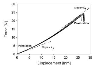
Fig. 6. Cook's knife stab test results from five experiments under 'reference' conditions, i.e., 4 mm thick skin with no underlying tissue and equi-biaxial tension of 10 N in both arms of the cruciform polyurethane skin simulants. Stab speed was 50 mm/min and blade was aligned perpendicular to skin (i.e., angle =  $0^{\circ}$ ). The dashed lines illustrate how initial and final tangent moduli for stiffnesses  $K_0$  and  $K_f$ , respectively are calculated.
