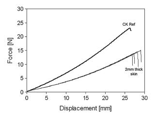
Fig. 9. Stab test results for the same cook's knife penetrating 4 mm (average of reference data in Fig. 6 shown above by single heavy line) and 2 mm (light lines represent four different tests) thick skin specimens. No underlying tissue was used; equi-biaxial tension of 10 N was applied; knife speed and orientation were 50 mm/min and  $0^{\circ}$ , respectively.
