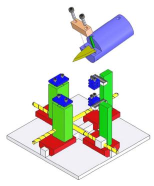
Fig. 4. Schematic of test arrangement showing (top) clamping of blade and (bottom) adjustable stage for clamping cruciform surrogate skin sample under biaxial tension with two pairs of clamps with load cells (seen immediately behind top right and bottom right clamps).
