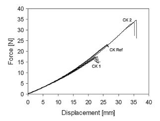
Fig. 7. Cook's knife stab test results under reference conditions: 4 mm thick skin specimens without underlying tissue under equi-biaxial tension of 10 N at 50 mm/min at 0°. The average of the reference data of Fig. 6 is shown by the single heavy line (labelled 'CK Ref'). Data from two sets of at least three tests using other new and nominally identical cook's knives are indicated by 'CK 1' and 'CK 2'.
