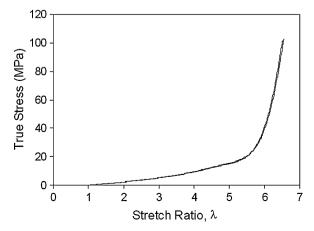
Fig. 2. True stress-stretch ratio data for longitudinal and transverse tests on skin simulant, polyurethane with Shore hardness 40A.
