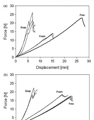
Fig. 13. Stab test results for (top) the same kitchen knife and (bottom) the same cook's knife ('CK 1' of Fig. 7) penetrating 4 mm thick skin specimens on top of different underlying tissue. Ballistic soap provides stiffer results than compliant foam, while the least stiff results occur in the absence of any underlying tissue. Equi-biaxial tension of 10 N was applied; knife speed and orientation were 50 mm/min and  $0^{\circ}$ , respectively.
