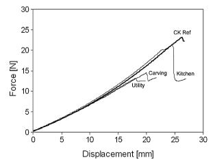
Fig. 8. Stab test results for all knives under reference conditions, i.e., 4 mm thick skin specimens,  $0^{\circ}$  angles of knife orientation, no underlying tissue, equibiaxial tension of 10 N; knife speed of 50 mm/min. The cook's knife (average of reference data in Fig. 6) is shown by heavy line whereas the utility, carving and kitchen knife curves are the average of at least three test repetitions each.
