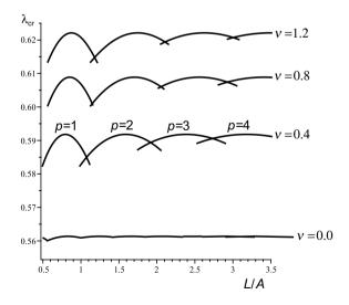
Fig. 6. Bending instability for a rectangular block with length-to-depth ratio  $L/(2A) \in [0.25, 1.75]$ . The neo-Hookean solid ( $\nu = 0.0$ ) can be bent more than solids with strain energy density (1), see plots at  $\nu = 0.4, 0.8, 1.2$ .
