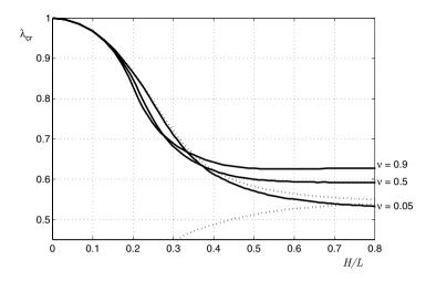
Fig. 4. Buckling of a compressed slab in plane-strain: critical stretch against H/L, the slab's initial slenderness. Solid curves: solids with strain energy density given by (1). Dashed curves: neo-Hookean solids.
