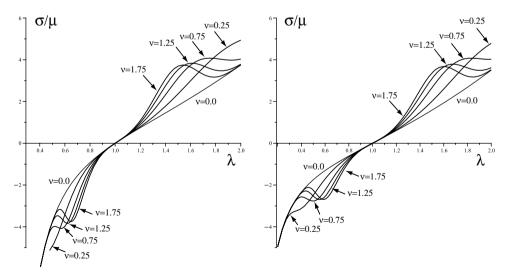
Fig. 1. Effect of localized strain-softening for the large deformations of solids with strain energy density given by (1). Stress–stretch curves in compression ( $\lambda < 1$ ) and in tension ( $\lambda > 1$ ), for plane-strain deformation (figure on the left) and uniaxial deformation (figure on the right), with  $\nu = 0$  (neo-Hookean solid), and  $\nu = 0.25, 0.75, 1.25, 1.75$ .
