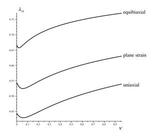
Fig. 3. Surface instability of a compressed solid with strain energy density given by (1). For uniaxial compression, plane-strain compression, and equibiaxial compression, the surface instability occurs earlier than for the neo-Hookean solid (which corresponds to  $\nu = 0$ ), once  $\nu > 0.15$ .
