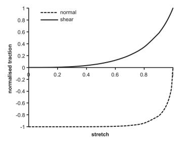
**Fig. 2.** Plots of the normal and shear components of the traction on slanted face versus  $\lambda_1$ .
