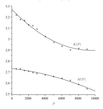
**Fig. 1.** Fit of the data measured by Hughes and Kelly [5] for pyrex subjected to hydrostatic pressure P (in bars) based on Eqs. (2.8) and (2.11) with  $\sigma = -P$  describing the large acoustoelastic effect: M and K are expressed in units of  $10^5$  bars.
