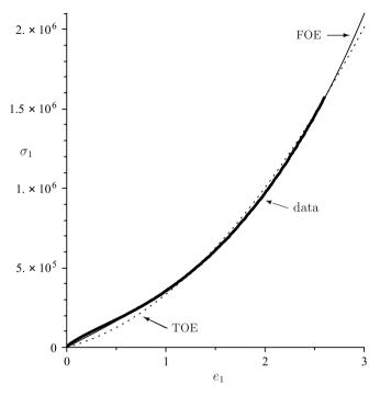
**Fig. 2.** Fitting tensile data (thick curve) of the Cauchy stress  $\sigma_1$  (in Pa) versus the elongation  $e_1$  for a sample of incompressible silicone rubber; the TOE strainenergy density cannot capture the variations adequately; the FOE model gives an excellent fit with only 3 material parameters, with values  $\mu=109.35$  kPa, A=-454.18 kPa, D=109.27 kPa.
