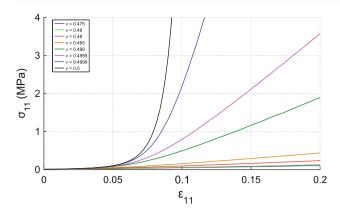
Fig. 2 Variation in Cauchy stress in 1-direction for different values of Poisson's ratio
