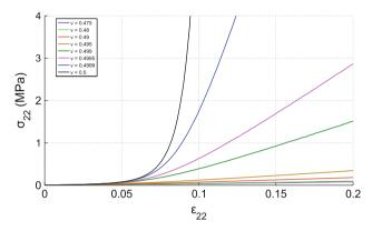
Fig. 3 Variation in Cauchy stress in 2-direction for different values of Poisson's ratio
