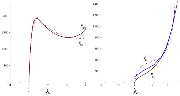
**Fig. 4.** Fitted pressure–stretch curves using the Mooney ( $P_M$ ) and the Gent–Gent ( $P_{GG}$ ) models for the inflation of a rubber balloon (left) and a monkey bladder. Blue curve: experimental data from [17] and [1]. (For interpretation of the references to color in this figure caption, the reader is referred to the web version of this paper.)
