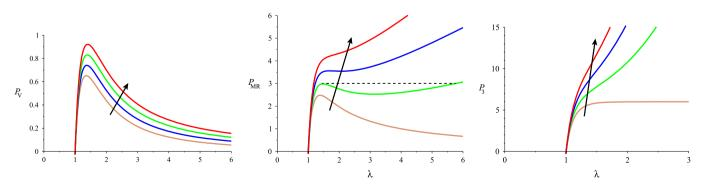
Fig. 2. Pressure–stretch curve for the inflation of a Mooney balloon. For the n=1 (Varga), n=2 (Mooney–Rivlin) and n=3 cases, the material parameter  $C_2/C_1$  takes the values 0.0, 0.1, 0.2, 0.3, as indicated by the arrows. Only the Mooney–Rivlin material (centre) can display both limit-point instability and inflation-point instability (see dashed horizontal line when  $C_2/C_1 = 0.1$ ).
