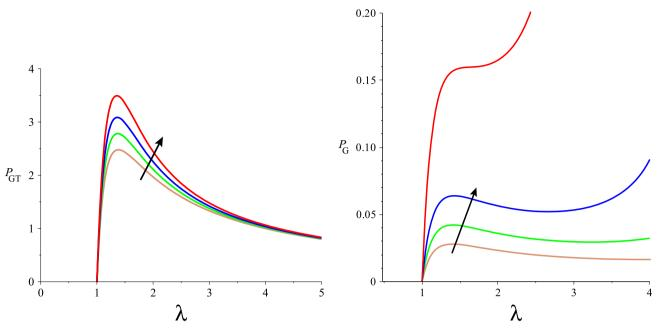
**Fig. 3.** Left: pressure–stretch curves for the inflation of a Gent-Thomas material, for the material parameters  $c_2/c_1 = 0.0, 0.3, 0.6, 1.0$  (increasing values indicated by the arrow); right: pressure–stretch curves for the inflation of a Gent material, for the stiffening parameters  $J_m = 90.0, 60.0, 40.0, 15.0$  (decreasing values indicated by the arrow).
