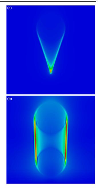
Fig. 1 Elastic Cerenkov effect induced by the moving point force in a soft material with the Mach number  $M_e = 3$ , (a); and b  $M_e = 30$ . For a large Mach number, the angle of the Mach cone is very small and the two quasi-plane shear waves form and propagate in opposite directions. The results are given by finite element analysis using an axisymmetric model
