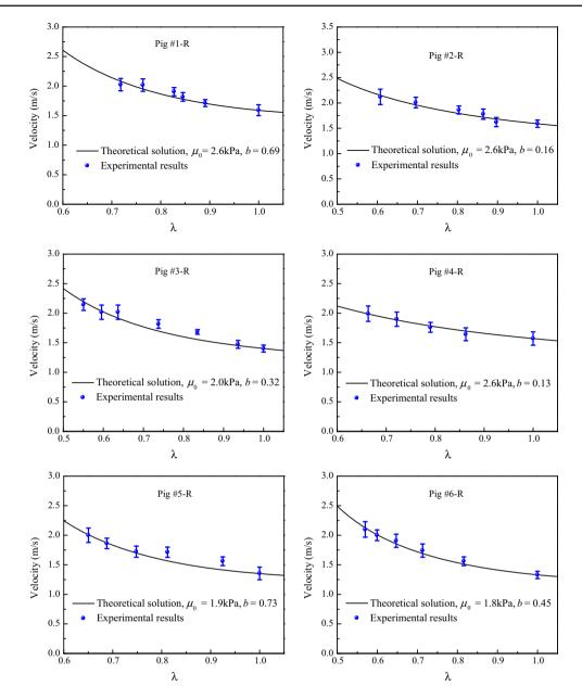
Fig. 5 Variation of the shear wave velocities with the compressive amount for the right lobes of the six different samples. The *error bars* show the standard deviation. The pre-strain parameter of tri-axiality  $\xi$  is taken as 0.5 according to the deformation of the tested material
