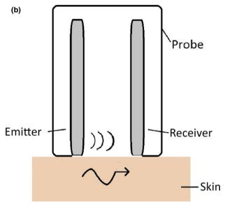
Fig. 1. (a) Reviscometer device<sup>®</sup>. (b) Mechanism of operation. [Colour figure can be viewed at wileyonlinelibrary.com]
