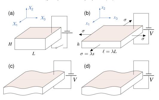
**Fig. 3.** When put under voltage V and/or stress  $\sigma$ , a rectangular plate made of a soft dielectric and with faces covered by compliant electrodes deforms homogeneously (a) and (b). It can even deform so severely as to lose its stability and buckle into antisymmetric (c) or symmetric (d) modes of wrinkles.
