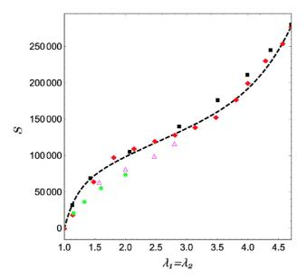
FIG. 1. Mechanical tuning of 3M VHB4905 in equibiaxial tension. Black squares taken from Ref. 4, and red diamonds refer to our own experiment. For information, we also give the stress-stretch pairs deduced from the voltage-stretch experiments of Ref. 7 (green circles) and Ref. 4 (magenta triangles) when the voltage is zero. The dashed curve indicates the best-fit function  $s(\lambda)$ .
