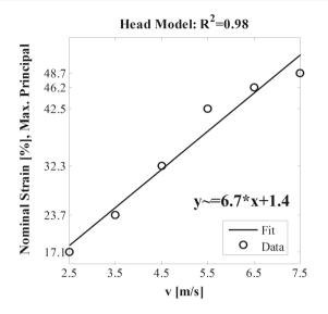
**Fig.4** Variation in the maximum principal value of the nominal strains [%] in the head model versus the speed impact values, v [m/s], used in the frontal head impacts of the head model. Linear regression fit also included
