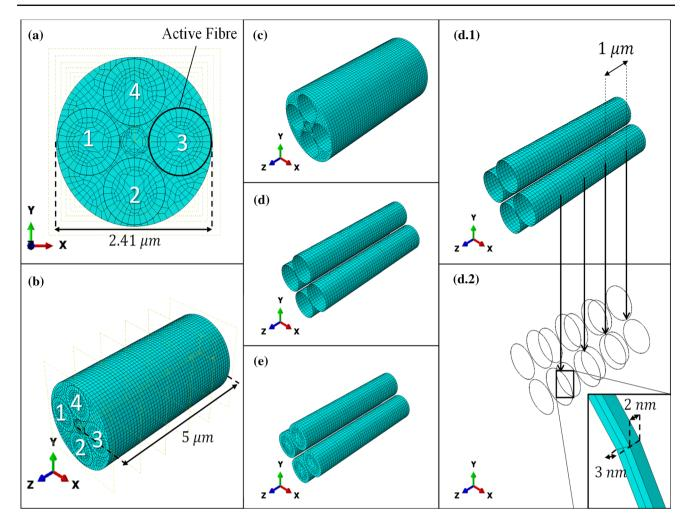
**Fig. 2 a** Frontal view and **b** isometric view of the three-layer nerve bundle made of four fibres. Fibre #3 is the active fibre, i.e. the fibre activated by a Gaussian voltage distribution (El Hady et al. 2015). Fibres #1, #2 and #4 are activated by the charges diffusing from Fibre #3. **c** the ECM; **d** the membrane; **e** the ICM. In the case of myelinated fibres, the membrane layer is periodically partitioned along the fibre length to model
