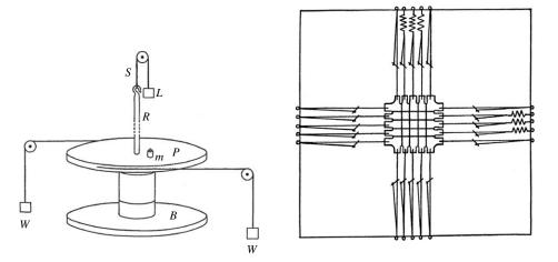
**Figure 2.** Rivlin was a very thorough and astute experimentalist. In one of his 10 articles published from 1948 to 1955 in *Philosophical Transactions*, he proposed protocols to measure the moment and normal force required to twist a rubber cylinder, and to measure stresses and strains in the bi-axial stretching of a rubber membrane [1].
