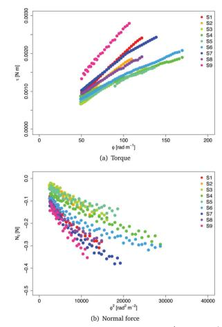
**Fig. 4** Results of the torsion tests performed at a twist rate  $\dot{\phi} = 300 \text{ rad m}^{-1} \text{ s}^{-1}$  on nine cylindrical samples of brain tissue excised from the coronal plane. (a) Torque  $\tau$  vs. twist  $\phi$  and (b) normal force  $N_z$  vs. twist squared  $\phi^2$ , measured for cylindrical samples with initial radius  $R_0 = 10$  mm.
