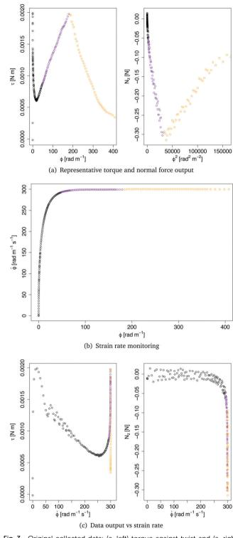
**Fig. 3** Original collected data: (a, left) torque against twist and (a, right) normal force against twist squared; (b) twist rate against twist; (c, left) torque and (c, right) normal force against twist rate. Black data: ramping towards the constant twist rate, see (b); purple: proper data of torsion; orange: data after breaking point, see (a).
