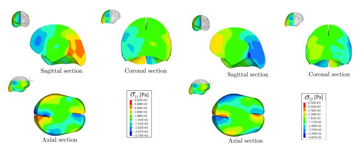
Figure 4: Results of the FE simulations of a rotational head impact, performed with the UCDBT Model. Distribution of the principal Cauchy stress components  $\sigma_{11}$  (on the left) and  $\sigma_{22}$  (on the right) in the Sagittal, Coronal and Axial planes. Here the orange and blue areas correspond to peak stress magnitude of approximatively 4 kPa, same as for the vertical stress component  $\sigma_{33}$ , see Figure 6 in the main paper.
