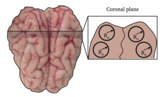
**Fig. 2** Sketch of the cutting map of a fresh porcine brain (top view). The cylindrical samples were obtained by cutting a slice of brain excised from the coronal plane into cylinders of radius  $R_0 = 10$  mm.
