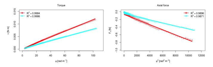
Figure 1: Torque and normal force data collected from the torsion tests at 12.5 radm<sup>-1</sup> for sample  $G_1$  (red) and  $G_2$  (cyan); and Mooney-Rivlin model prediction (solid lines).
