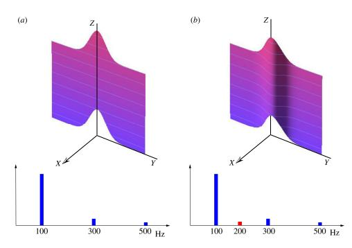
**Figure 2.** Sketches of the Gaussian beams in §3: (*a*) a pure anti-plane shear Gaussian beam generates only odd harmonics, at 100, 300, 500 Hz, while (*b*) an initially noisy Gaussian beam (with a small in-plane component) additionally generates a harmonic at 200 Hz. (Online version in colour.)
