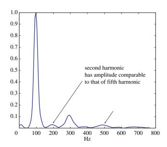
**Figure 1.** Spectrum generated by a large shear excitation in gelatine: experimental results of Espíndola *et al.* [15] (shared by G. Pinton and D. Espíndola). (Online version in colour.)
