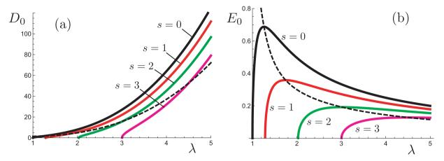
**Fig. 1.** Plots of (a)  $D_0$  versus  $\lambda$  and (b)  $E_0$  versus  $\lambda$  based on  $E_0$ . (31)<sub>1</sub> and the connection  $E_0 = \lambda^{-4}D_0$  for the neo-Hookean dielectric in equi-biaxial deformation, for values of non-dimensional pre-stress s = 0, 1, 2, 3 (continuous curves). In (a) we also display the (dashed) curve of  $D_0 = \sqrt{(\lambda^6 + 5)/3}$ , the intersections of which with the continuous curves correspond to the maxima in (b).
