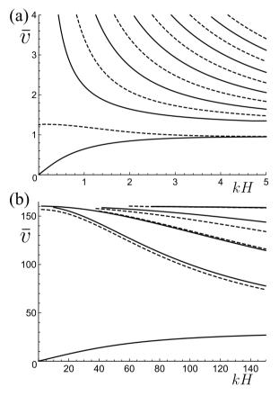
**Fig. 9.** The non-dimensionalised Lamb wave speed  $\bar{v} = v\sqrt{\rho/\mu}$  against *kH* of antisymmetric and symmetric modes shown by solid and dashed curves, respectively, for a Gent electroelastic plate with no pre-stress ( $\bar{T} = 0.0$ ). (a) The response at the snap-through point where  $\bar{E}_{max} = 0.689$  and  $\lambda = 1.264$ , and (b) The past snap-through point where  $\bar{E}_{max} = 0.689$  and  $\lambda = 6.926$ , see Fig. 6.
