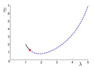
**Fig. 8.** The dimensionless velocity  $\bar{v}$  of the fundamental symmetric mode in the long wavelength-thin plate limit ( $kH \rightarrow 0$ ) against the stretch  $\lambda$  for a Gent electro-elastic plate. The wave speed marked by ' $\bullet$ ' occurs when  $\lambda = 1.264$  and  $\bar{E}_0 = \bar{E}_{max} = 0.689$ .
