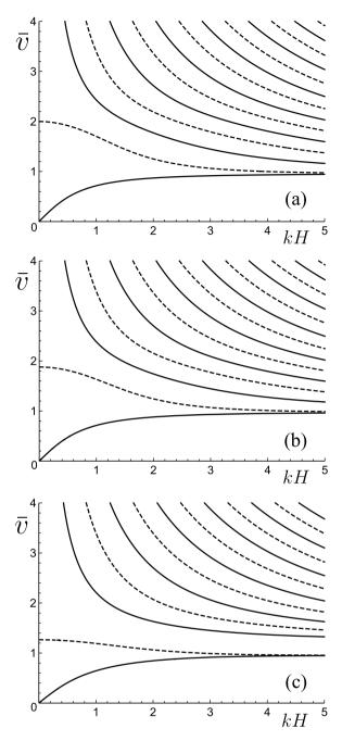
**Fig. 2.** The dimensionless Lamb wave speed  $\bar{v} = v \sqrt{\rho/\mu}$  against *kH* of antisymmetric and symmetric modes shown by solid and dashed curves, respectively, for a neo-Hookean electroelastic plate with  $\bar{T} = 0$ . (a) Purely elastic un-stretched case  $\bar{E}_0 = 0, \lambda = 1$ , (b) Moderate electrical loading  $\bar{E}_0 = 0.4, \lambda \simeq 1.03$ , and (c) Maximal electrical loading  $\bar{E}_0 = \bar{E}_{max} = \sqrt{3}/2^{4/3}, \lambda = 2^{1/3}$ .
