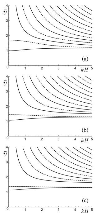
**Fig. 5.** The dimensionless wave speed  $\bar{v} = v \sqrt{\rho/\mu}$  against *kH* of antisymmetric (solid) and symmetric (dashed) modes for a pre-stressed neo-Hookean electroelastic plate, with  $\bar{T} = 0.8$ . (a) The elastic case with  $\bar{E}_0 = 0, \lambda \simeq 1.2$ , (b) Moderate electric field  $\bar{E}_0 = 0.4, \lambda \simeq 1.4387$ , and (c) The maximal electric field  $\bar{E}_0 \simeq 0.4148, \lambda \simeq 1.5916$ .
