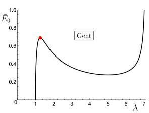
**Fig. 6.** The loading curve  $\bar{E}_0$  against the in-plane stretch  $\lambda$  for a Gent electro-elastic plate with  $J_m = 97.2$  and  $\bar{T} = 0$ .
