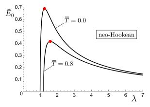
**Fig. 1.** The loading curve  $\bar{E}_0$  against the in-plane stretch  $\lambda$  for a neo-Hookean electroelastic plate with no pre-stress ( $\bar{T} = 0.0$ , upper curve) and with pre-stress  $\bar{T} = 0.8$  (lower curve). The field  $\bar{E}_0$  increases initially with increasing values of  $\lambda$ , obtains its maximum  $\bar{E}_{max}$  (marked by ' $\bullet$ ') and decreases afterwards. As the pre-stress increases,  $\bar{E}_{max}$  decreases, see [13] for a detailed discussion.
