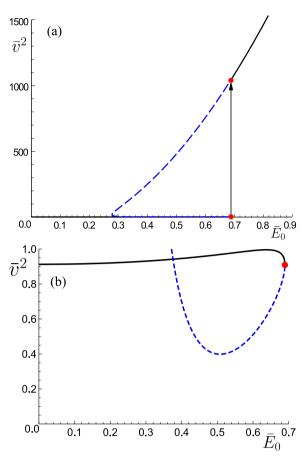
**Fig. 7.** The dimensionless Rayleigh wave speed  $\bar{v}^2$  against  $\bar{E}_0$  for a Gent electroelastic plate with no pre-stress ( $\bar{T} = 0.0$ ) in the short wavelength-thick plate limit. (a) The jump in velocity due to snap-through. (b) The Rayleigh wave speed before the snap-through instability. The values of  $\bar{v}^2$  corresponding to  $\bar{E}_0 = \bar{E}_{max} = 0.689$  are denoted by ' $\bullet$ '.
