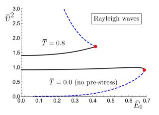
**Fig. 4.** The dimensionless squared Rayleigh wave speed  $\bar{v}^2 = \rho v^2 / \mu$  against  $\bar{E}_0$  for a neo-Hookean electroelastic plate with  $\bar{T} = 0.0$  and  $\bar{T} = 0.8$ , and  $kH \to \infty$  (short wavelength-thick plate limit). The wave speed  $\bar{v}^2$  when  $\bar{E}_0 = \bar{E}_{max}$  for each case is again marked by '•'.
