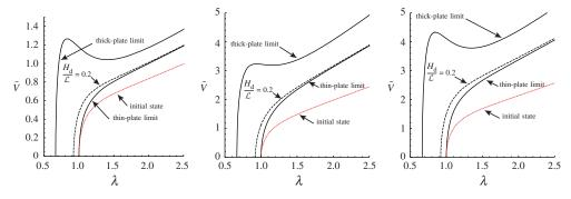
**Figure 6.** Dependence of the non-dimensional electric potential  $\bar{V}$  on the in-plane stretch  $\lambda$  for values of  $\bar{\varepsilon}=0.3, 0.6$  and  $\bar{H}=0.3, 0.8$ . Specifically, the panel on the left shows the wrinkling behaviour and the initial state for  $\bar{\varepsilon}=0.3, \bar{H}=0.3$ , the centre panel corresponds to  $\bar{\varepsilon}=0.6, \bar{H}=0.3$  and the results on the right to  $\bar{\varepsilon}=0.6, \bar{H}=0.8$ . (Online version in colour.)
