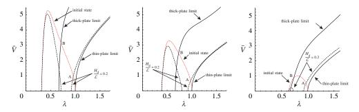
**Figure 8.** The panel on the left shows the initial state and the dependence of the non-dimensional electric potential  $\bar{V}$  on the in-plane stretch  $\lambda$  for values of  $\bar{\varepsilon}=1.5$  and  $\bar{H}=0.3$ . The panel in the centre is obtained when  $\bar{\varepsilon}=2$  and  $\bar{H}=0.3$  and the results on the right correspond to  $\bar{\varepsilon}=2$  and  $\bar{H}=0.8$ . (Online version in colour.)
