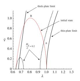
**Figure 7.** The  $\bar{V}-\lambda$  loading curves and the initial state of an immersed neo-Hookean electro-elastic plate for permittivity and thickness ratios  $\bar{\varepsilon}=2$  and  $\bar{H}=0.8$ , respectively. The solid curves depict the behaviour for the thin- and thick-plate limits, the dashed curve corresponds to  $H_{\rm d}/\mathcal{L}=0.2$  and the dotted red curve represents the initial state when  $\bar{s}=0$ . (Online version in colour.)
