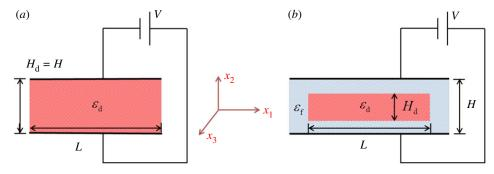
**Figure 1.** Loading scenarios for an electro-elastic plate. In (*a*) the electric field is generated by a potential difference between two flexible electrodes coated on the main faces; in (*b*) the plate is immersed in a tank filled with silicone oil with the electric field generated by two rigid electrodes placed at the top and bottom of the tank. (Online version in colour.)
