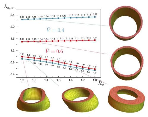
**Fig. 7.** Distribution of residual stress after growth subject to an external electric field  $\bar{V} = 0.4, 0.6$  and axial stretch  $\lambda_z$ . The integer values given in the neighbourhood of each point are the couple  $n_{cr}$ ,  $m_{cr}$ .
