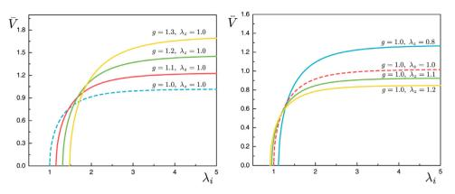
**Fig. 4.** The effect of the growth factor g and axial stretch  $\lambda_z$  on the nonlinear response of inner circumferential stretch  $\lambda_i$  versus the applied voltage  $\bar{V}$ , in the case  $\bar{R}_o = 2.0$ .
