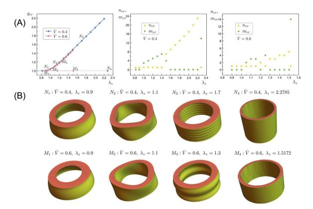
**Fig. 9.** (A) The influence of the external axial strain on the critical growth factor and the corresponding wave numbers with applied voltage  $\bar{V} = 0.4$ , 0.6, where  $\bar{R}_0 = 1.4$ ,  $R_i = 1.0$ , L = 1.0; (B) some typical patterns of (A).
