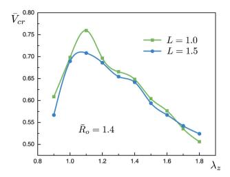
**Fig. 8.** The effect of axial stretch on the critical voltage with  $\bar{R}_0 = 1.4$  and L = 1.0, 1.5.
