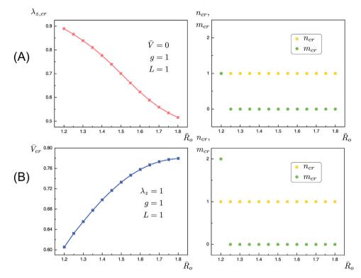
**Fig. 6.** Tube of length L = 1.0. (A) Critical axial stretch  $\lambda_{z,cr}$  and modes of instability  $m_{cr}$ ,  $n_{cr}$ , when there is no growth (g = 1.0) and no voltage applied ( $\bar{V} = 0.0$ ). (B). Critical voltage  $\bar{V}_{cr}$  and modes of instability when there is no growth (g = 1.0) and no axial stretch ( $\lambda_z = 1.0$ ).
