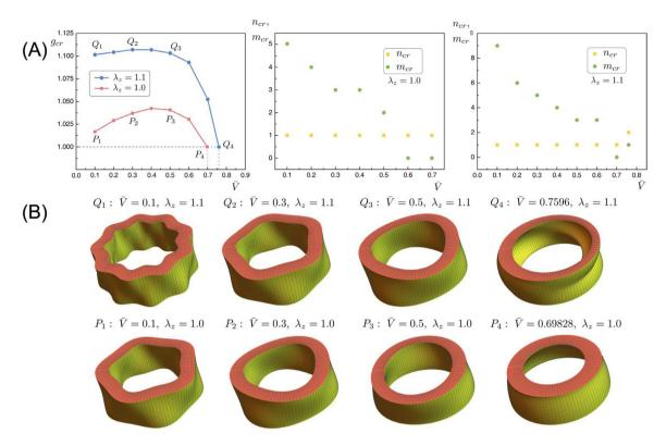
**Fig. 10.** (A) The influence of the applied voltage on the critical growth factor and the corresponding wave numbers with axial stretches  $\lambda_z = 1.0, 1.1$ , where  $\tilde{R}_0 = 1.4, R_i = 1.0, L = 1.0$ ; (B) some typical patterns of (A).
