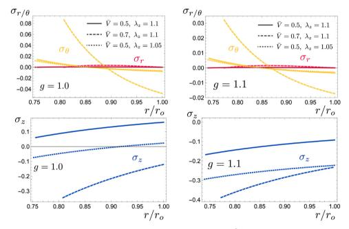
Fig. 5. The distribution of residual stress of a tube that subjects to the external electric field  $\bar{V}$  and axial stretch  $\lambda_z$  after growth, where  $\bar{R}_0 = 2.0$ .
