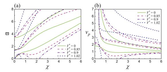
**Fig. 14.** Frequency spectra (a) and phase velocity spectra (b) of the first three modes of the L waves in a functionally graded SEA tube with  $\beta_i = 2.0$  (i = 1, ..., 4) and  $\lambda_z = 1.0$ , for different values of  $V^*$ .
