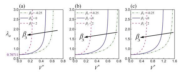
**Fig. 5.** Variations of the inner surface circumferential ratio  $\lambda_a$  with the dimensionless voltage  $V^*$  in a functionally graded SEA tube with  $\lambda_z = 2.0$  and  $\Delta P^* = 0$ , for different permittivity gradients  $\beta_3$  and three sets of elastic moduli gradients: (a)  $\beta_1 = \beta_2 = -0.25$ ; (b)  $\beta_1 = \beta_2 = 0$ ; (c)  $\beta_1 = \beta_2 = 2.0$ .
