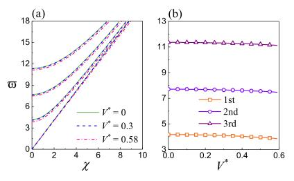
**Fig. 10.** (a) Frequency spectra of the first four modes of the T waves for different values of  $V^*$ , and (b) the first three nonzero cut-off frequencies at  $\chi = 0$  versus  $V^*$  in a functionally graded SEA tube with  $\beta_i = 2.0$  (i = 1, ..., 4) and  $\lambda_z = 2.0$ .
