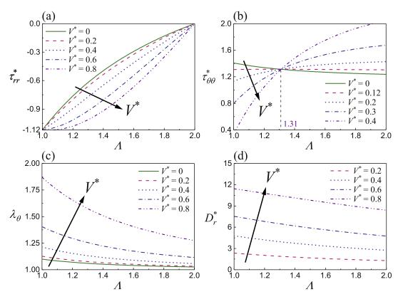
**Fig. 7.** Radial distributions of the dimensionless radial normal stress  $\tau_{rr}^*$  (a), circumferential normal stress  $\tau_{\theta\theta}^*$  (b), circumferential stretch  $\lambda_{\theta}$  (c), and radial electric displacement  $D_r^*$  (d) in a functionally graded SEA tube with  $P_{out}^* = 0$ ,  $P_{inn}^* = 1.12$ ,  $\lambda_z = 1.0$  and  $\beta_1 = \beta_2 = \beta_3 = 5.0$ , for different values of  $V^*$ .
