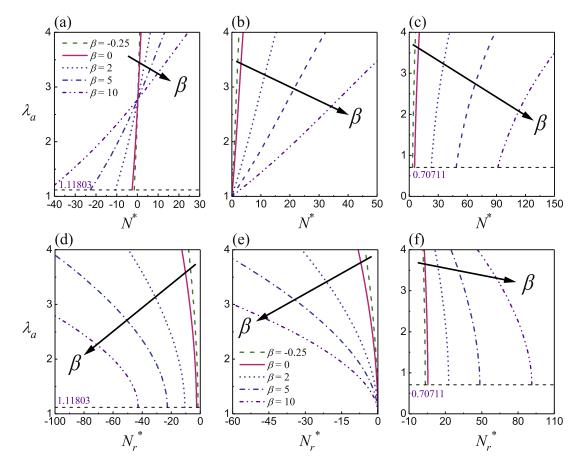
**Fig. 6.** Variations of the inner surface circumferential ratio  $\lambda_a$  with the dimensionless *resultant* axial force  $N^*$  (a-c) and *reduced* axial force  $N^*_r$  (d-f) in a functionally graded SEA tube with  $P^*_{out} = 0$  and  $V^* = 0$ , for different material gradients  $\beta = \beta_1 = \beta_2 = \beta_3$  and various axial pre-stretches  $\lambda_z$ : (a, d)  $\lambda_z = 0.8$ ; (b, e)  $\lambda_z = 1.0$ ; (c, f)  $\lambda_z = 2.0$ .
