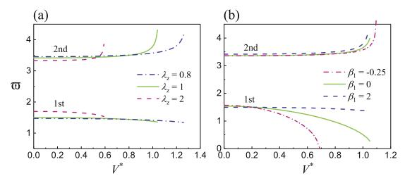
**Fig. 15.** The first two nonzero cut-off frequencies at  $\chi = 0$  of the L waves versus  $V^*$ : (a) for different axial pre-stretches  $\lambda_z$  (with  $\beta_i = 2.0$ , i = 1, ..., 4); (b) for different material gradients  $\beta = \beta_i$  (i = 1, ..., 4) (with  $\lambda_z = 1.0$ ).
