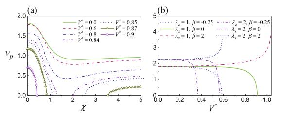
**Fig. 16.** (a) Phase velocity spectra of the lowest L wave mode in a *homogeneous* ( $\beta_i = 0, i = 1, ..., 4$ ) SEA tube with  $\lambda_z = 1.0$  for different values of  $V^*$ . (b) Variations of the lowest L wave phase velocity at  $\chi = 0$  with  $V^*$  for different combinations of the axial pre-stretch  $\lambda_z$  and material gradient  $\beta = \beta_i$  (i = 1, ..., 4).
