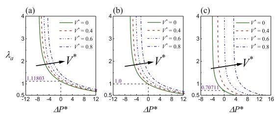
**Fig. 3.** Variations of the inner surface circumferential ratio  $\lambda_a$  with the dimensionless pressure difference  $\Delta P^*$  in a functionally graded SEA tube with material gradient  $\beta = \beta_1 = \beta_2 = \beta_3 = 5.0$ , for different values of voltage  $V^*$  and various axial pre-stretches  $\lambda_z$ : (a)  $\lambda_z = 0.8$ ; (b)  $\lambda_z = 1.0$ ; (c)  $\lambda_z = 2.0$ .
