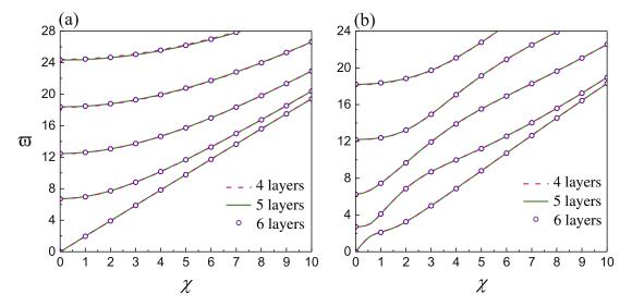
**Fig. 9.** Convergence analysis of frequency spectra of the first five wave modes obtained by the SSM for a functionally graded SEA tube with  $\beta_1 = \beta_2 = 5.0$ ,  $\beta_3 = \beta_4 = 1.0$ ,  $\lambda_z = 1.0$  and  $V^* = 0.2$ : (a) T waves; (b) L waves. Here n = 4, 5, 6 is the number of the discretized thin layers.
