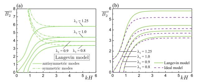
**Fig. 8.** Uni-axial loading for four fixed values of pre-stretch  $\lambda_1=0.8,0.9,1.0,1.25$ : (a) critical magnetic induction field  $\overline{B}_2^{cr}$  as a function of kH for antisymmetric (solid lines) and symmetric (dashed-dotted lines) modes of the neo-Hookean saturation Langevin plates; (b)  $\overline{B}_2^{cr}$  as a function of kH for antisymmetric modes of the neo-Hookean ideal (dashed lines) and saturation Langevin (solid lines) magneto-elastic plates.
