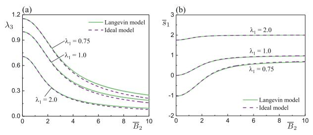
Fig. 3. Uni-axial loading for three different values of pre-stretch  $\lambda_1=0.75, 1.0, 2.0$ : (a) response of the stretch ratio  $\lambda_3$  versus the dimensionless magnetic induction field  $\overline{B}_2$  from Eq. (75)<sub>2</sub>; (b) response of the dimensionless nominal mechanical traction  $\overline{s}_1$  versus  $\overline{B}_2$  from Eq. (75)<sub>1</sub>. Solid lines correspond to the ideal magneto-elastic model while dashed lines represent the saturation Langevin model.
