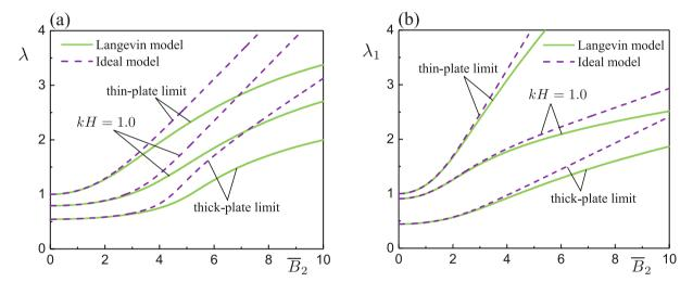
**Fig. 4.** Bifurcation curves (or critical combinations of stretch ratio and dimensionless magnetic induction field) of antisymmetric wrinkling modes for the thin- and thick-plate limits and kH = 1.0: (a) plane-strain loading ( $\lambda$  versus  $\overline{B}_2$ ); (b) uni-axial loading ( $\lambda_1$  versus  $\overline{B}_2$ ). Solid lines correspond to the ideal magneto-elastic model while dashed lines represent the saturation Langevin model.
