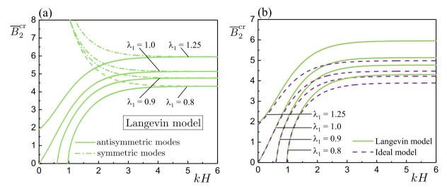
**Fig. 7.** Plane-strain loading for four fixed values of pre-stretch  $\lambda=0.8,0.9,1.0,1.25$ : (a) critical magnetic induction field  $\overline{B}_2^{cr}$  as a function of kH for antisymmetric (solid lines) and symmetric (dashed-dotted lines) modes of the neo-Hookean saturation Langevin plates; (b)  $\overline{B}_2^{cr}$  as a function of kH for antisymmetric modes of the neo-Hookean ideal (dashed lines) and saturation Langevin (solid lines) magneto-elastic plates.
