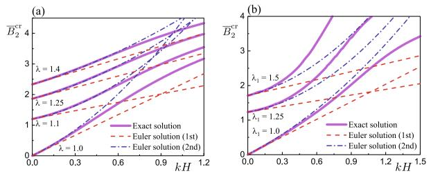
**Fig. 10.** Critical magnetic induction field  $\overline{B}_2^{cr}$  as a function of kH for antisymmetric modes of a neo-Hookean ideal magneto-elastic plate subject to different fixed pre-stretch: (a) plane-strain loading with  $\lambda = 1.0, 1.1, 1.25, 1.4$ ; (b) uni-axial loading with  $\lambda_1 = 1.0, 1.25, 1.5$ . The solid lines, dashed lines, and dashed-dotted lines represent, respectively, the exact solutions, the first-order and second-order Euler buckling solutions.
