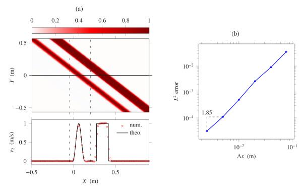
Fig. 2. Linear initial-value problem with initial data consisting of a smooth sinusoidal bump and a rectangular bump. (a) Top: map of the velocity  $v_2$  in m/s obtained numerically. Bottom: cut along the line Y = 0. (b)  $L^2$  error measurements restricted to the line segment between dashed lines.
