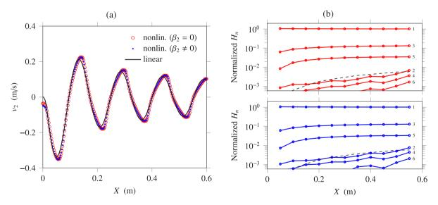
**Fig. 6.** Nonlinear boundary-value problem with purely cubic nonlinearity (red), or with quadratic and cubic nonlinearity (blue). (a) Velocity signal obtained numerically at  $t \approx 0.6$  s; (b) Normalized harmonic amplitudes with respect to the propagation distance if  $\beta_2 = 0$  (top) or if  $\beta_2 \neq 0$  (bottom). The dashed curve marks the fifth harmonic obtained in the linear case (Fig. 5b).
