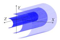
Fig. 1. Typical directional wave fields of this study; Sketch of equal-phase surfaces issued from a line source located on the Z-axis.
