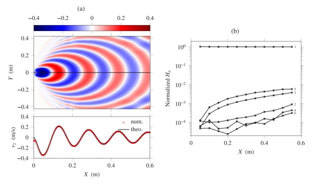
**Fig. 5.** Linear boundary-value problem. (a) Top: snapshot of the velocity  $v_2$  at  $t \approx 0.6$  s; Bottom: numerical and analytical solutions along the line Y = 0. A video of the simulation is provided in the supplementary material. (b) Evolution of the normalized harmonic amplitudes with the propagation distance X at Y = 0 (labels: order n).
