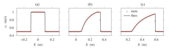
**Fig. 4.** Nonlinear initial-value problem (27) which is invariant along the Y-direction. Numerical and analytical solution displayed at t = 0 s (a), t = 0.1 s (b) and t = 0.2 s (c).
