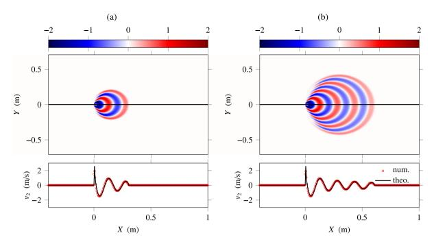
**Fig. 3.** Linear non-homogeneous problem with initial data consisting of a sinusoidal point source. Top: map of the velocity  $v_2$  in m/s obtained numerically at  $t \approx 0.2$  s (a) and  $t \approx 0.4$  s (b). Bottom: comparison of the numerical and analytical solutions along the line Y = 0.
