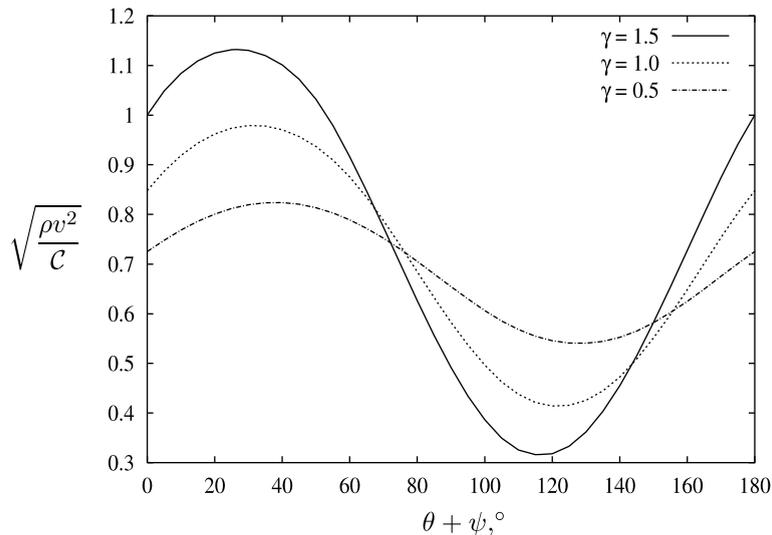
Fig. 5. Scaled surface wave speed as a function of  $\theta + \psi$  for a Varga material subjected to simple shear deformations.
