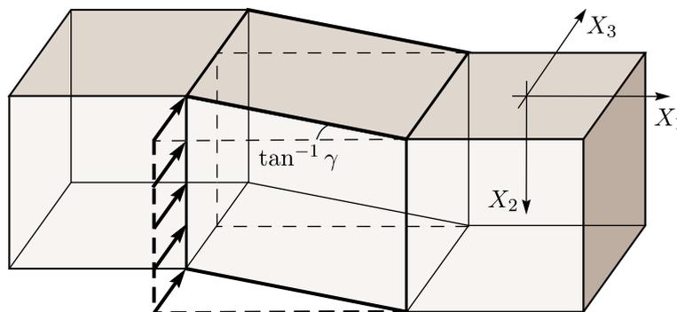
Fig. 4. An elastic material under simple shear; the dashed lines represent the body at rest.
