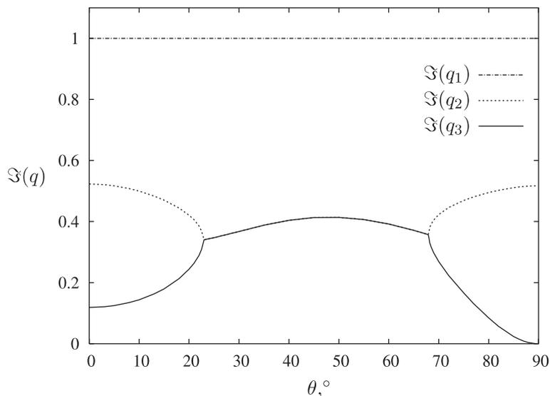
Fig. 3. Imaginary part of the attenuation coefficients for a surface wave in a deformed Mooney–Rivlin material.
