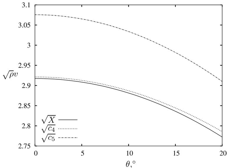
Fig. 2. Scaled speeds of bulk and surface waves near the direction of greatest stretch in a Mooney–Rivlin material.
