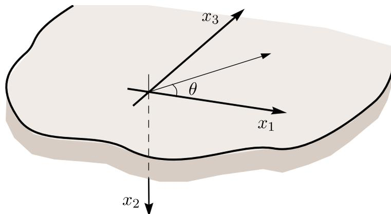
Fig. 1. A surface wave propagating in a principal plane but not in a principal direction.
