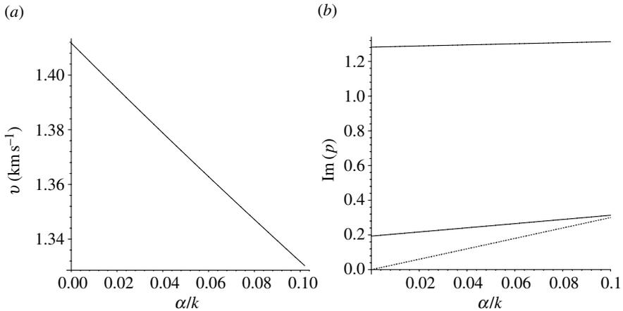
Figure 1. Exponentially graded orthotropic shales: variations with the dispersion parameter  $\alpha/k$  of (a) the surface wave speed and (b) the imaginary parts of the quantities  $p_1$  and  $p_2$  appearing in equation (2.14) (the dashed line is the plot of  $3\alpha/k$ , above which  $\text{Im}(p_1)$ ,  $\text{Im}(p_2)$  must be for the wave to decrease faster than the inhomogeneity).
