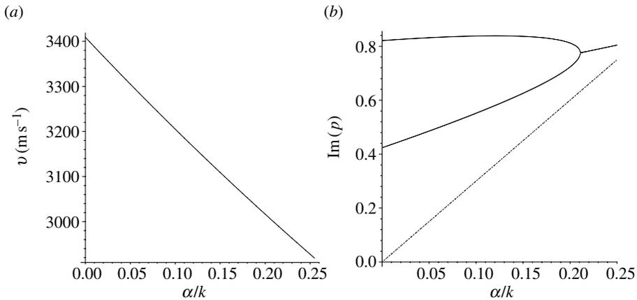
Figure 2. Exponentially graded silica: variations with the dispersion parameter  $\alpha/k$  of (a) the surface wave speed and (b) the imaginary parts of the quantities  $p_1$  and  $p_2$  appearing in equation (2.14) (the dashed line is the plot of  $3\alpha/k$ ).
