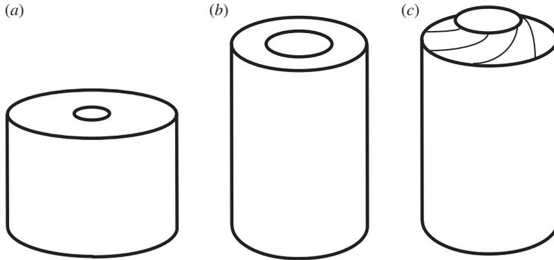
Figure 1. (a) Shrink fit of an elastic tube, followed by the combination of (b) simple torsion and (c) helical shear. (The figure is not drawn to scale among the various deformations.)
