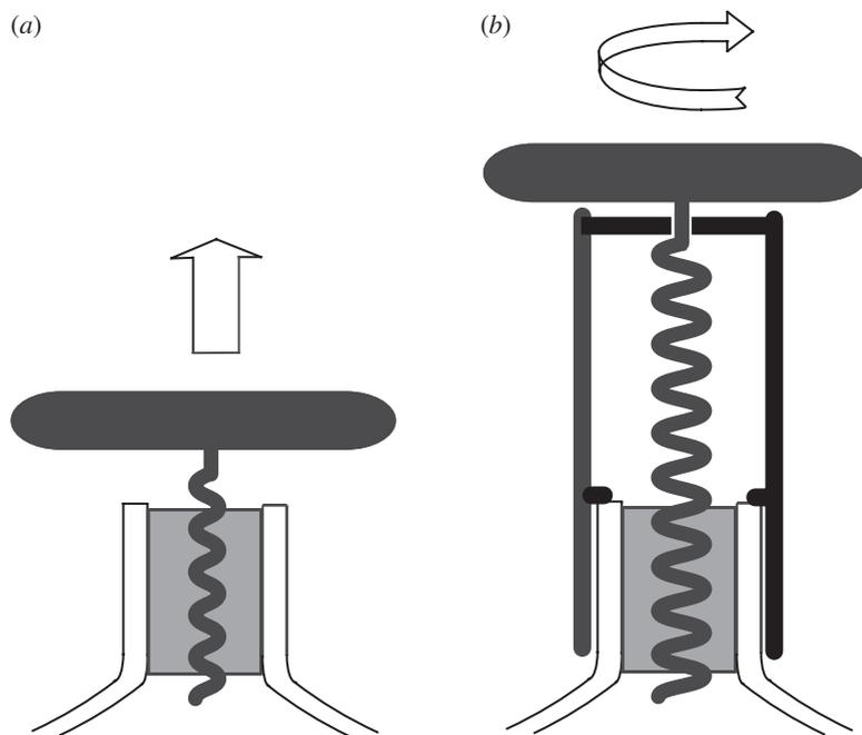
Figure 4. There are two main types of corkscrews: (a) one that relies on pulling only and (b) another that adds a twist to the cork-pulling action. The analysis developed in this paper indicates that the second type is more efficient.
