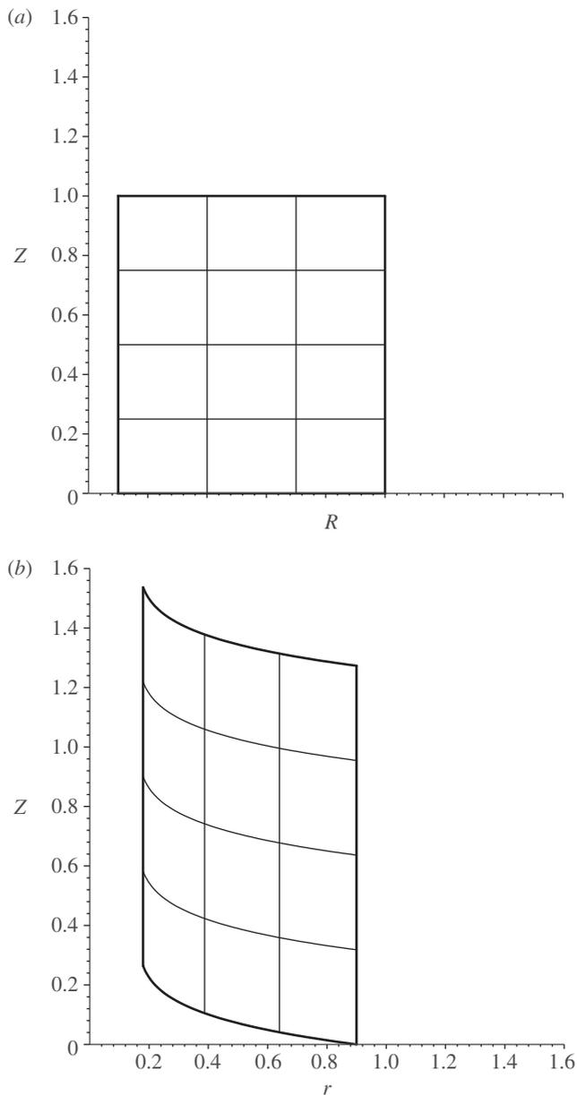
Figure 2. (a,b) Pulling on the inside face of a neo-Hookean tube. Here the vertical axis is the symmetry axis of the tube.
