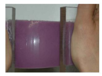
**Fig. 1.** Bending a block of silicone, until creases appear on the inner face. Here the block has dimensions  $16.5 \text{ cm} \times 5 \text{ cm} \times 6 \text{ cm}$ , giving an aspect ratio L/A = 3.36. The end faces of the block were glued onto plexi-glass plates, and these are subjected manually to a bending moment. At least three axial wrinkles are visible.
