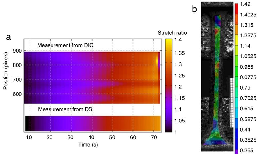
**Fig. 7 – (a) Comparison of stretch measurement from DIC and DS over the length of the specimen throughout the duration of a given tensile test. (b) Distribution of local Lagrangian strains just before rupture. Note the area of localized magnification in red. This is the location where rupture subsequently occurred.**
