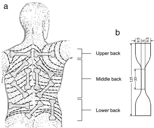
**Fig. 1 - (a) Orientation of samples from the back. Specimens are superimposed onto a map of the Langer lines to indicate their orientation with respect to the lines (Langer, 1861). (b) Dimensions of custom made dye (mm).**
