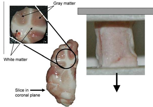
Fig. 2. Extraction of cylindrical specimens containing mixed white and gray matter (left). Specimen in stretched position after test (right).
