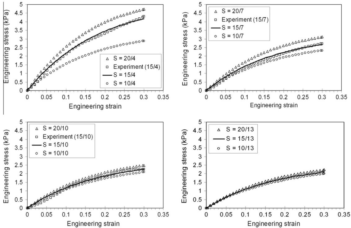
Fig. 6. Variation in engineering stress profiles at different aspect ratios,  $S = \text{diameter/thickness}$ .
