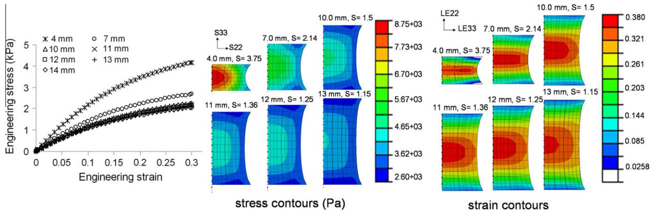
Fig. 5. Stress and strain contours at variable specimen thicknesses, at a maximum stretch ratio of 1.3. Left figure shows decrease in magnitude of engineering stress (Pa) with increasing specimen thickness (4–14 mm). Middle figures show that significantly higher stresses are evident for specimens of 4 mm thickness. Right figures show that a homogeneous strain field is evident for specimen thicknesses of 10mm and greater, i.e.,  $S \leq 1.5$ .
