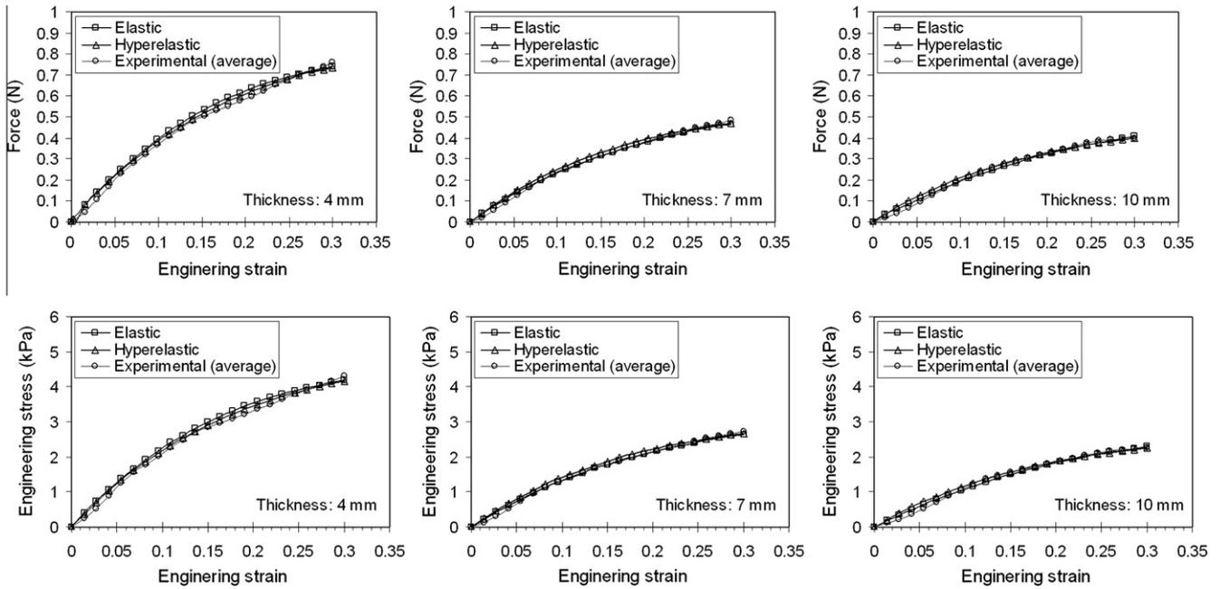
Fig. 4. Excellent agreement of elastic, hyperelastic and experimental stress (kPa) and force (N) profiles at different sample thicknesses, using Ogden material parameters ( $\mu = 4395.0$  Pa,  $\alpha = -2.8$ ) and Young's modulus  $E = 11200$  Pa (at 10% strain).
