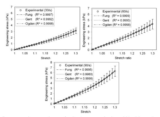
Fig. 6 – Excellent agreement between strain energy functions (Fung, Gent and Ogden models) and the experimental nominal stress is achieved at 30, 60 and 90/s strain rates (p=0.9990).
