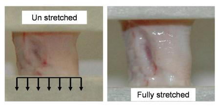
Fig. 4 – Cylindrical brain specimen ( $10.0\pm0.1$  mm) fully stretched to achieve 30% strain. Arrows indicate downward movement of the lower platen producing stretch in the brain tissue at a specific strain rate.
