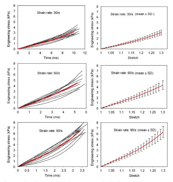
Fig. 5 – Tensile tests performed on porcine brain tissue up to 30% strain at loading velocity of 300 mm/s (strain rate: 30/s), 600 mm/s (strain rate: 60/s) and 900 mm/s (strain rate: 90/s).
