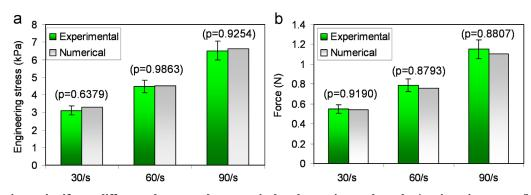
Fig. 9 – There is no significant difference between the numerical and experimental results (engineering stress (kPa) and force (N)) based on one way ANOVA tests.
