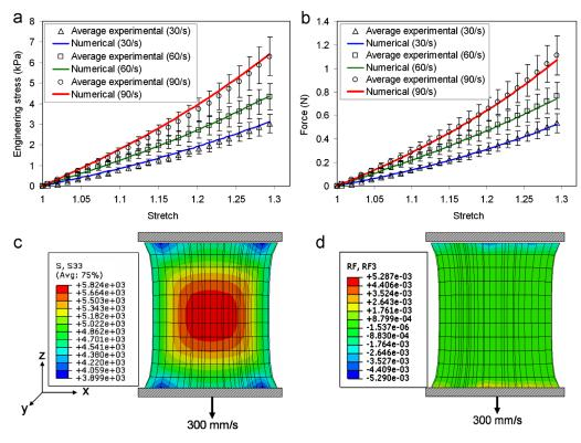
Fig. 8 – Simulations showing numerical stress and reaction force contours (a) agreement of experimental and numerical engineering stresses (kPa) at each strain rate, (b) agreement of experimental and numerical forces (N) at each strain rate, (c) cross-sectional view showing stress contours (Pa) at 30% strain and (d) cross-sectional view showing reaction force contours (N) at 30% strain.
