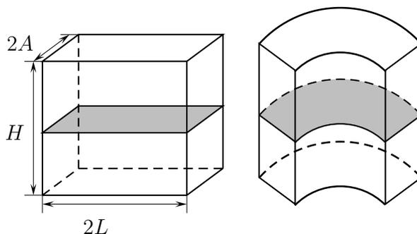
Figure 1: Cylindrical bending of a rubber block
