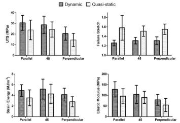
Fig. 2: Effect of sample orientation at dynamic strain rates (N=33, 14.5-29 s<sup>-1</sup>) and at quasi static strain rates (N=55,  $0.83 \text{ s}^{-1}$ ).
