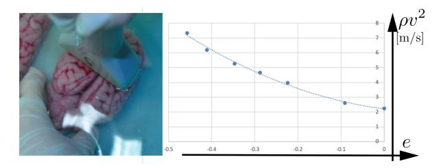
Figure 2: Using acousto-elasticity to find the material parameter of an intact pig brain. The curve fitting exercise on the right yields  $\mu = 2.2$ , A = -15.0, D = 8.7 kPa.
