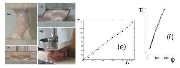
Figure 1: Standard testing protocols for soft solids applied to brain matter (porcine): (a) tensile test with glued ends and (b) compression test with lubricated faces: notice the inhomogeneity of the resulting deformations; (c) simple shear and (d) torsion: here the samples behave as required for the modelling. (e): shear stress Vs amount of shear [1]; (f): torque Vs twist [2].
