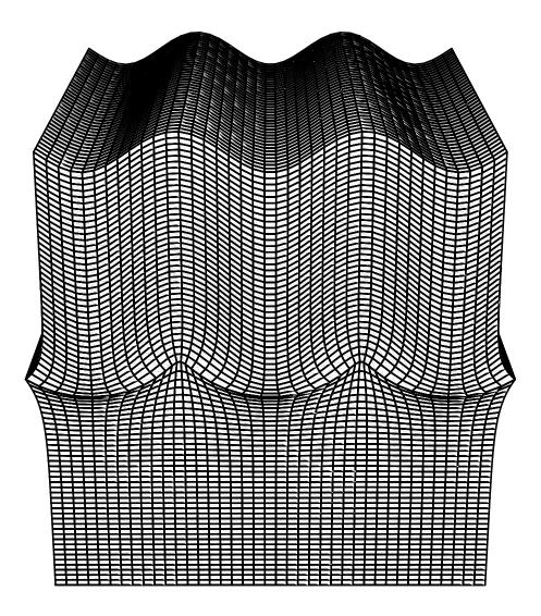
Figure 10: Displacements due to a Stoneley wave at the interface between Nickel (top) and Silica (bottom). Its amplitude decays exponentially with distance from the interface. The Stoneley wave speed (2921 m/s) is very close to the speed of the bulk shear wave in Nickel (2922 m/s), which is why the decay occurs over much greater distances in the upper half-space than in the bottom one.
