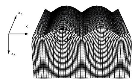
Figure 6: A Rayleigh surface wave in a homogeneous semi-infinite solid with Poisson ratio  $\nu = 1/4$ . Its amplitude decays exponentially with depth and is polarized in the sagittal plane (which includes the direction of propagation  $x_1$ and the normal to the boundary  $x_2$ ). The ellipse of polarization is described in a retrograde manner near the surface.
