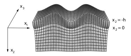
Figure 8: Displacements due to a Love surface wave in a superficial layer with shear modulus  $\hat{\mu}$  and mass density  $\hat{\rho}$ , rigidly bonded to a semi-infinite substrate with shear modulus  $\mu = 2\hat{\mu}$  and mass density  $\rho = \hat{\rho}$ . Here the wave propagates with a wavelength which is 4 times h, the layer thickness, and only the fundamental mode exists.
