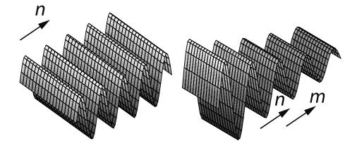
Figure 1: Homogeneous waves. On the left: a wave with constant amplitude; On the right: a wave with an attenuated amplitude.
