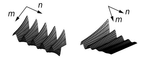
Figure 2: Inhomogeneous waves. On the left: the planes of constant phase are orthogonal to the planes of constant amplitude; On the right: they are at  $45^{\circ}$ .
