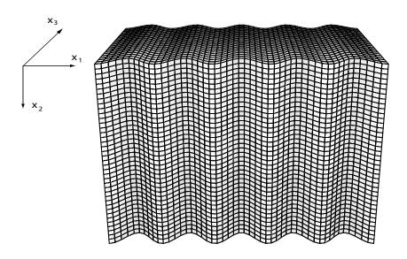
Figure 4: A shear horizontal surface wave in a homogeneous semi-infinite solid. It propagates in the  $x_1$ -direction, and is polarized in the  $x_3$ -direction. Its amplitude remains constant with the depth  $x_2$ . It is unlikely to be observed at all.
