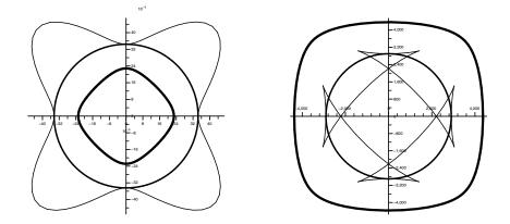
Figure 3: Homogeneous bulk waves in a plane of symmetry for copper (cubic symmetry). On the left: slowness surface (s/m); On the right: wavefronts, represented by the group velocity (m/s). Values used:  $d_{11} = 17.0$ ,  $d_{12} = 12.0$ ,  $d_{44} = 7.5$  (10<sup>10</sup> Pa), and  $\rho = 8.9 \times 10^3$  (kg/m<sup>3</sup>).
