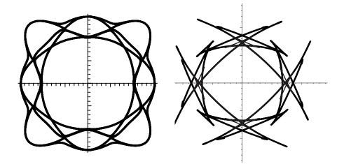
Figure 9: Surface waves in a plane of symmetry for Copper (cubic symmetry). On the left: slowness surface; On the right: wavefronts.
