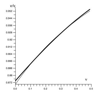
Figure 5: The speed of a Rayleigh wave in an isotropic solid with Poisson ratio  $\nu$ . Thick curve: numerical solution to the exact equation; Thin curve: approximate solution using the formula  $v/v_T \simeq (0.87 + 1.12\nu)/(1 + \nu)$ .
