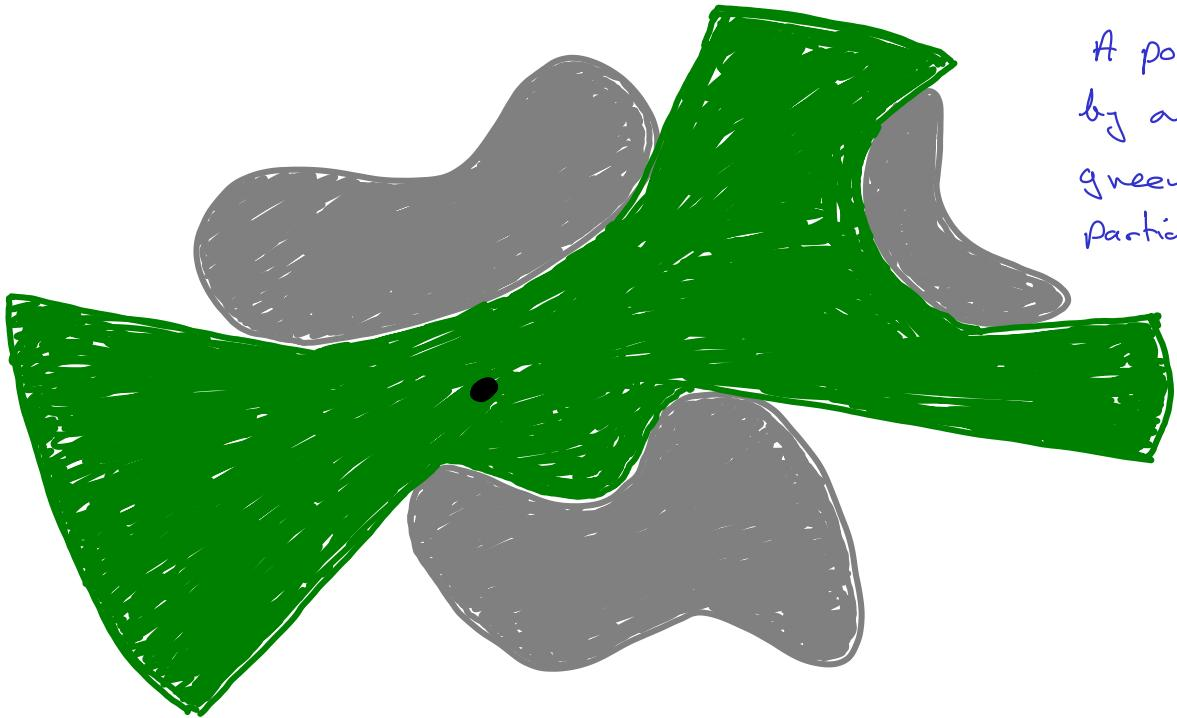
A point can is detected by all sensors in the green area; it is partially hidden by the grey objects.
